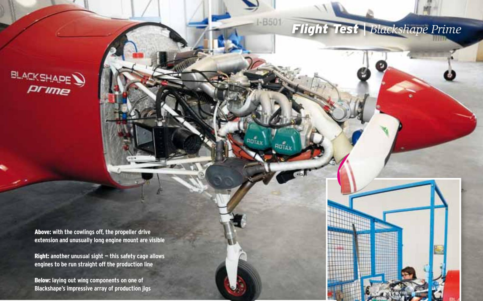
Above: with the cowlings off, the propeller drive extension and unusually long engine mount are visible
